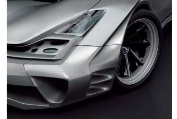
A lightweight PP compound with improved impact resistance is used for bumpers and other components.
